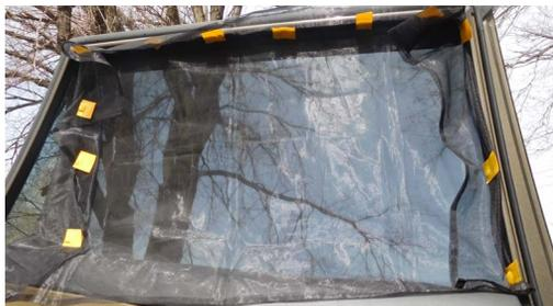
Figure 3. The screen and magnets placed inside a window frame.
