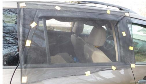
Figure 1. The screen and magnets placed on the outside of a vehicle. (Note that the magnets are lighter in color to improve visibility in the photos.)
