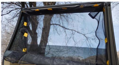
Figure 4. If you can't secure the bottom of the screen with magnets, it is helpful to keep the screen tight between the side magnets and to keep the window rolled up a few inches (8 cm.).
