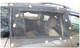
Figure 1. The screen and magnets placed on the outside of a vehicle. (Note that the magnets are lighter in color to improve visibility in the photos.)
